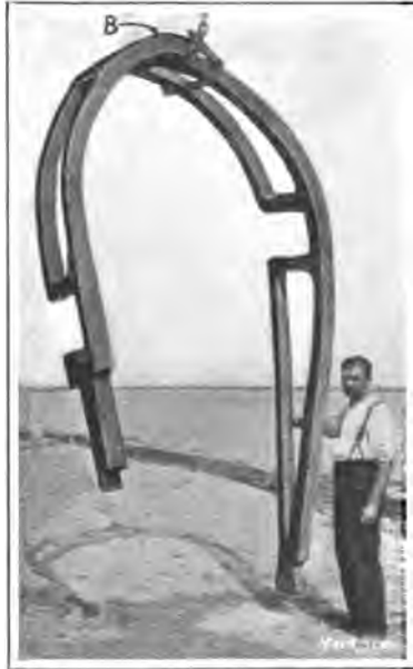
Fig. 4. Locomotive Frame bent to Test Quality of Steel Casting
